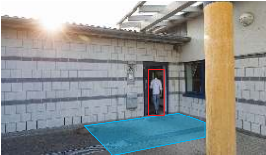
The "Intrusion Detection" analytic triggers an alarm when a person enters the restricted area.
